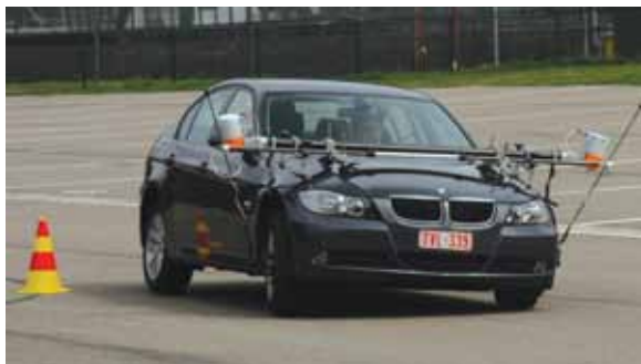
Slalom test for wheel behavior analysis
