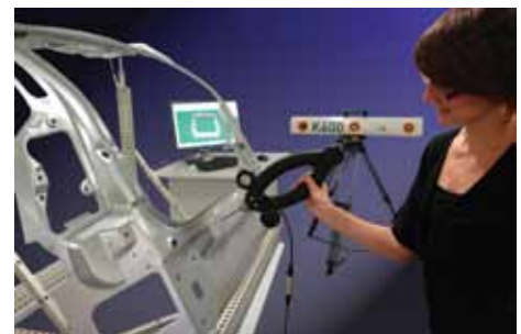
K-Series Optical CMM with SpaceProbe for large volume measurements
