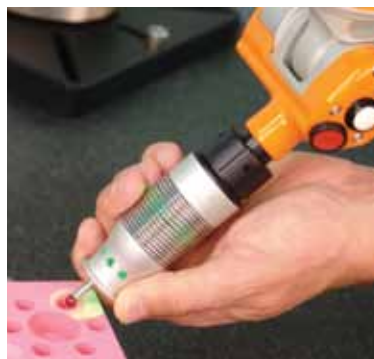
MCA comes in 6 or 7-axis versions for touch trigger or laser scanner measurement
