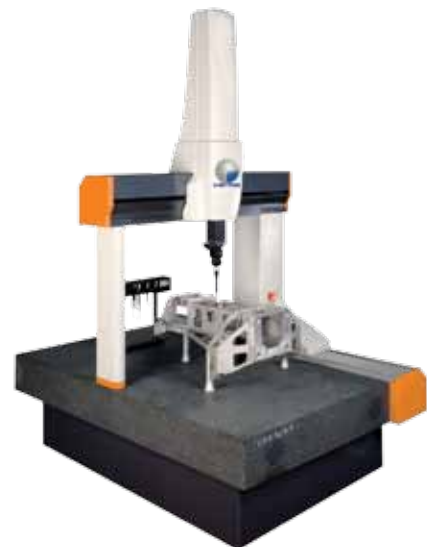
C3 bridge CMMs are high-specification, cost effective metrology solutions
