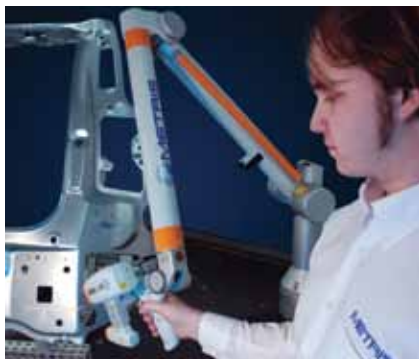
MCA comes in 6 or 7-axis versions for touch trigger or laser scanner measurement
